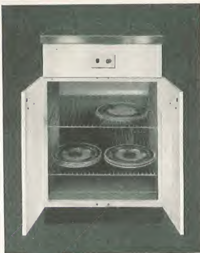
Plate warmer cabinet has satin finish chromium steel lining, is insulated with rock-wool and electrically heated. The cabinet is equipped with two woven wire sliding shelves.
